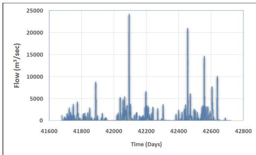
**Fig. 9 (b)** Flash Floods Graph for GSMaP Dataset Generated by HEC-HMS.
